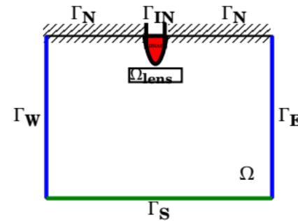
Abbildung: Geometry and boundary conditions for the DNAPL infiltration problem
