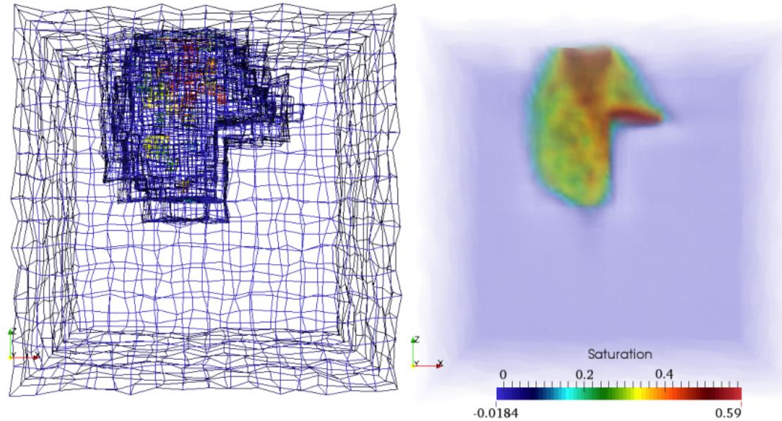
Abbildung: 3d-Problem: Saturation distribution after 3000 s of injection with  $0.25 \text{ Kg s}^{-1}\text{m}^{-2}$  of DNAPL. Unstructured mesh. Polynomial order  $p = 1$ .
