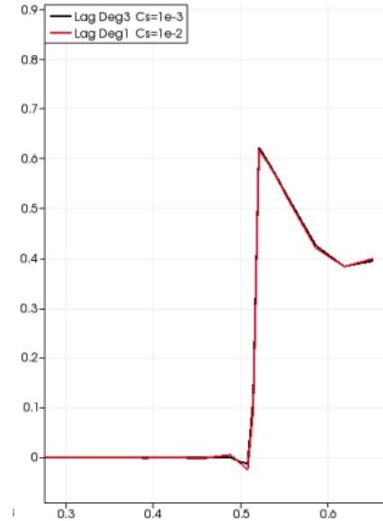
Abbildung: Comparison of non-wetting-phase saturation at  $T=2000$  s. Left, profile along the line  $((0,0);(0.45,0.65))$ . Right, profile along the line  $x=0.45$  m.
