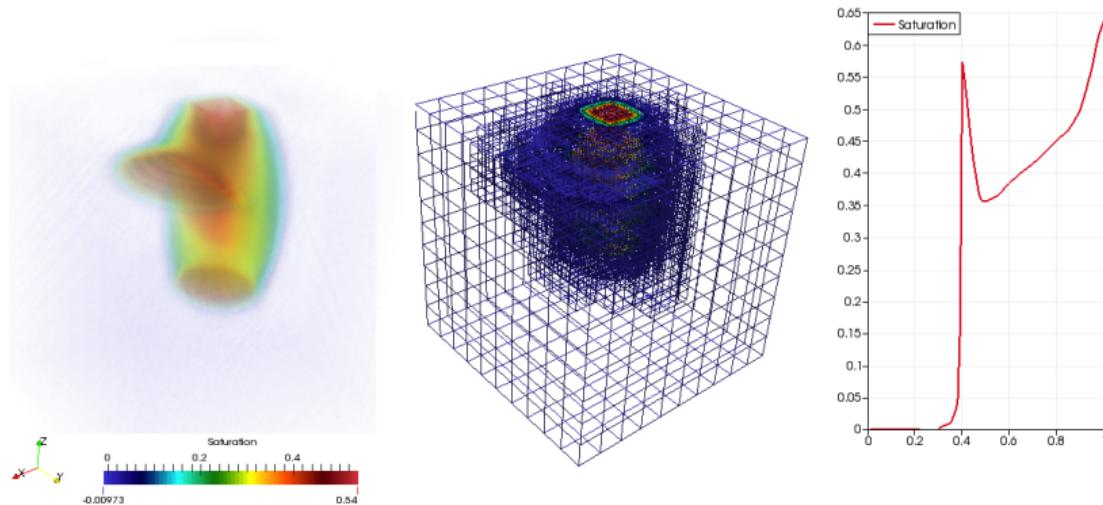
Abbildung: Contour plot of saturation distribution after 3600 s of injection with  $0.25 \text{ Kg s}^{-1}\text{m}^{-2}$  of DNAPL in a depth of 1 m (left column), leaf grid (center column) and saturation profile along the line ((1,0.45,0);(0.45,0.45,1))(right column).
