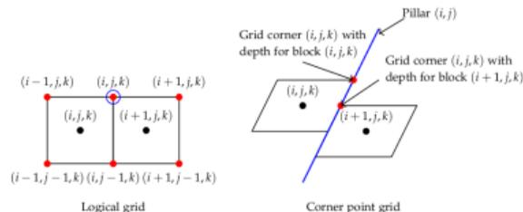
for different grid cells, as illustrated in the right figure in Fig. 7.6. Each logical corner in the regular  $i, j, k$  grid is shared by 8 grid cells. Different depths for the same logical corner can be used for representing faults and non-reservoir gaps.
